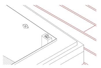
The comfort roof exit has a limit switch for opening monitoring on the opposite narrow side of the exit, as well as a light barrier for monitoring the exit area of the element.
