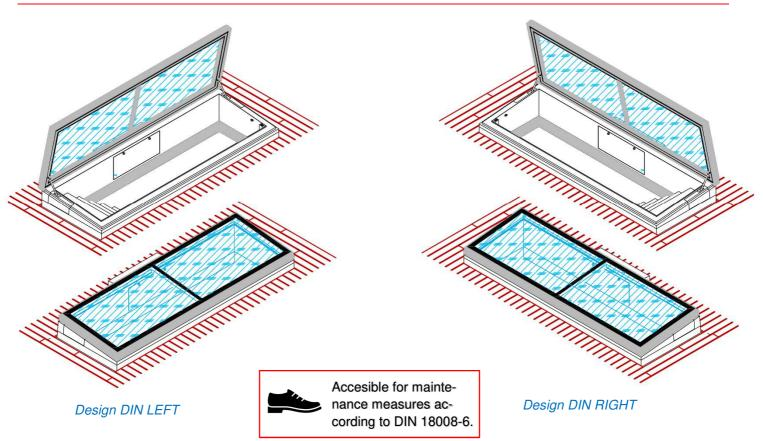
The LAMILUX Flat Roof Exit Comfort Swing consists of a thermally seperated, high-strength aluminium connection system, a fully insulated core bonded zone as well as a circumferential double-sealing system.
