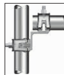
Use of the lattice beam coupler
