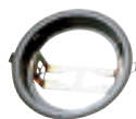
Installation ring for 5" loudspeaker For 9329.1 loudspeaker. For mounting in hollow walls/ceilings. With spring brackets. Drilling measurements: 160 mm. Mounting depth: 110 mm.
