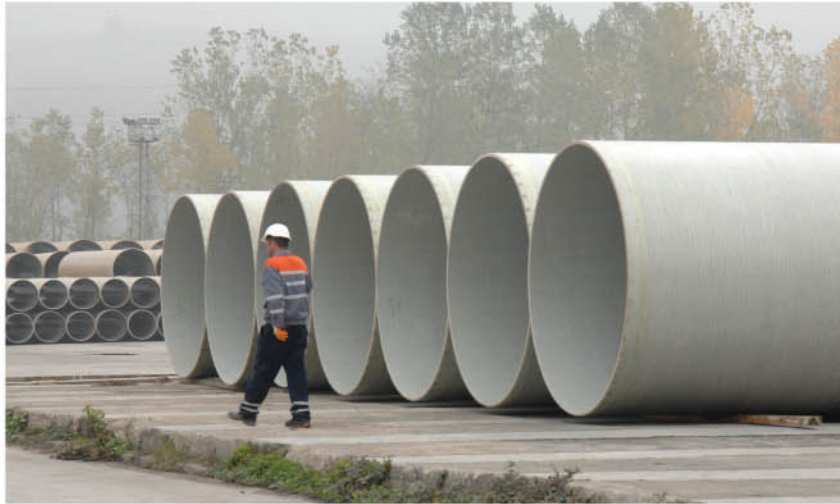
Figure 4 : Storage of pipes as a single level
