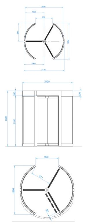
Concrete Base to specification at least (cube) 30N/mm2 of resistance. Base to be flat and level to +/-5mm over footprint area. Dimensions to be >2250 x 2250 x 150 deep min. (units in mm).
