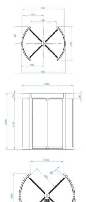
Concrete Base to specification at least (cube) 30N/mm2 of resistance. Base to be flat and level to +/-5mm over footprint area. Dimensions to be > 2250 x 2250 x 150 deep min. (units in mm).
