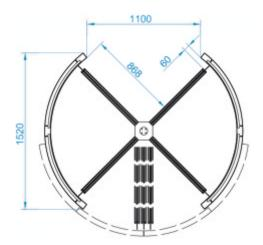
Concrete Base to specification at least (cube) 30N/mm2 of resistance. Base to be flat and level to +/-5mm over footprint area. Dimensions to be >  $2050 \times 2050 \times 150$  deep min. (units in mm).
