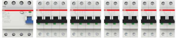
I1-3 HPFI-A 40A30mA + 1x4P 16A-C + 2x2P 10A-C + + 1HPFI-A 40A30mA + 1x4P 16A-C + 2x2P 10A-C
